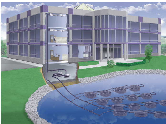
Figure 33: Surface Water Loop Application
